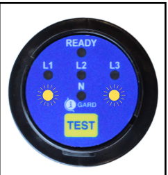
Figure 5.3.b: Flashing AMBER LEDs
