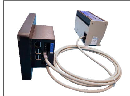
Figure 7: SIGMA3-C and TDM connection
