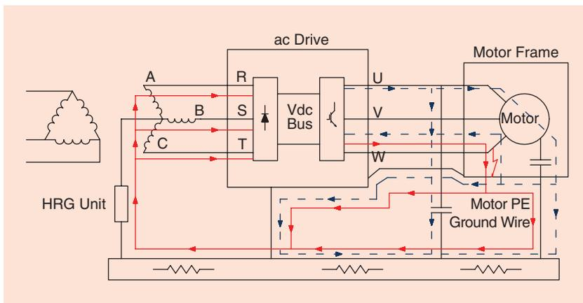
**FIGURE 12.** A UPS or ASD indicating a common mode current due to a switching supply and a zero sequence due to a ground fault at the motor.
