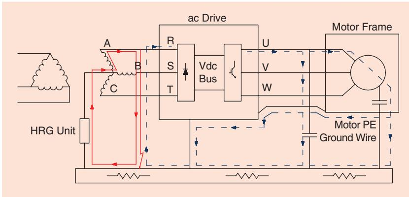
**FIGURE 9.** A UPS or ASD indicating a common mode current due to the switching supply and a zero sequence due to a ground fault on the line side.
