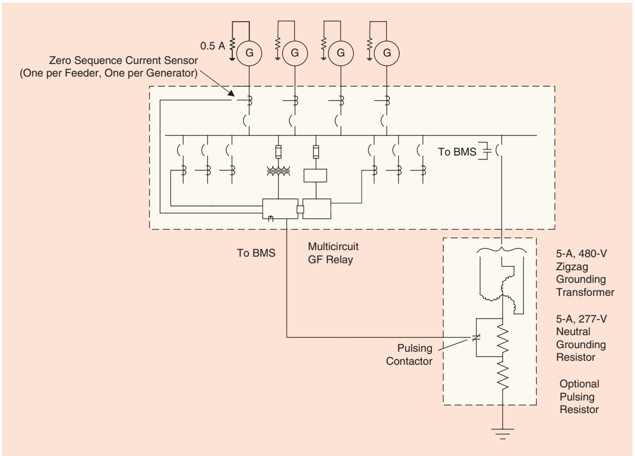
**FIGURE 6.** The HRG at the main bus. BMS: building management system.
