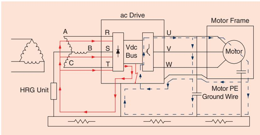
**FIGURE 10.** A UPS or ASD indicating a common mode current due to the switching supply and a zero sequence due to a ground fault on the dc link.
