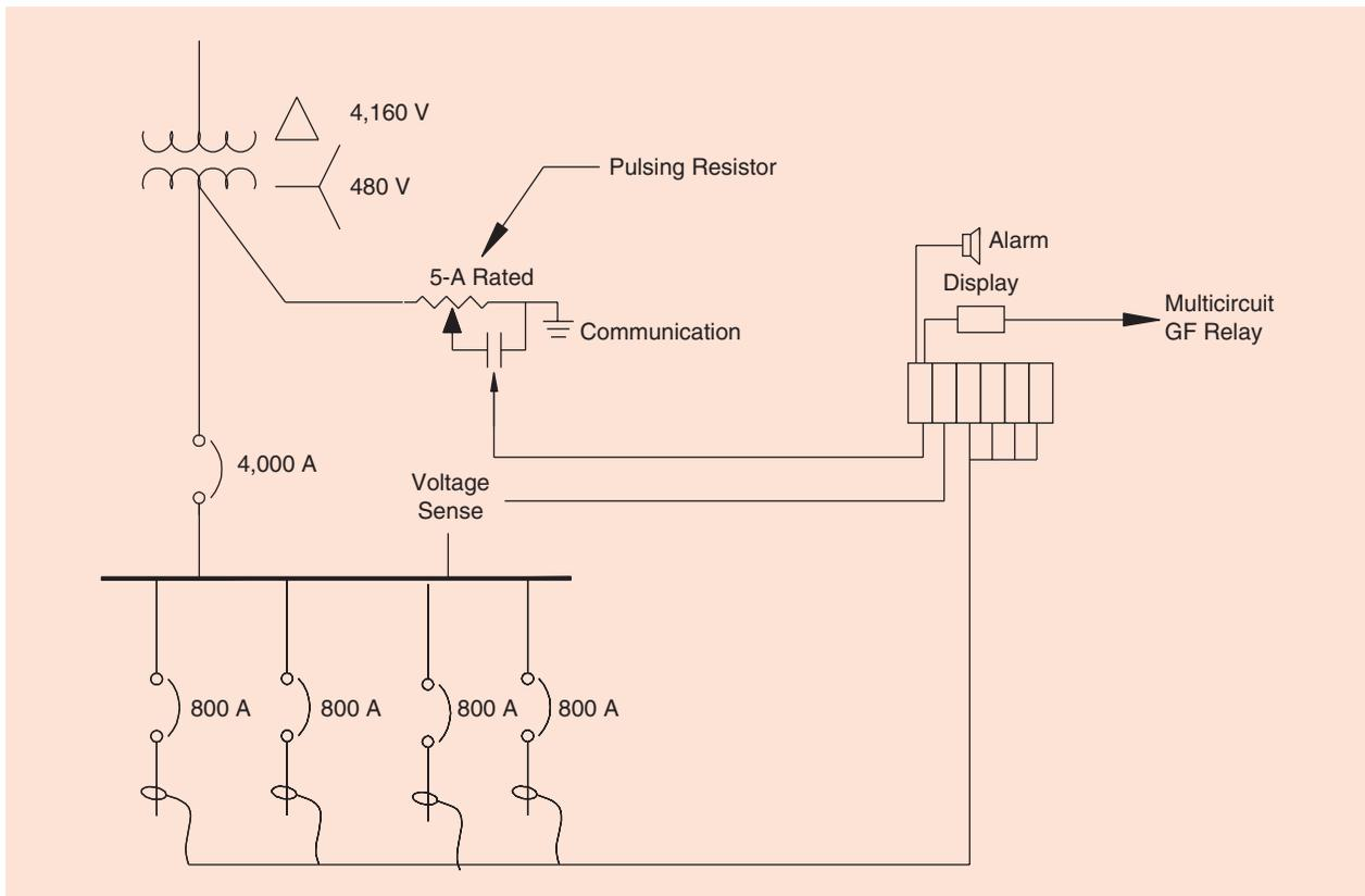
**FIGURE 1.** A typical delta/bye installation. GF: ground fault.
