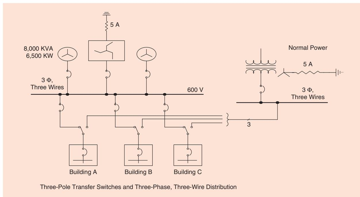
**FIGURE 5.** A standby generator and three-pole transfer switches.
