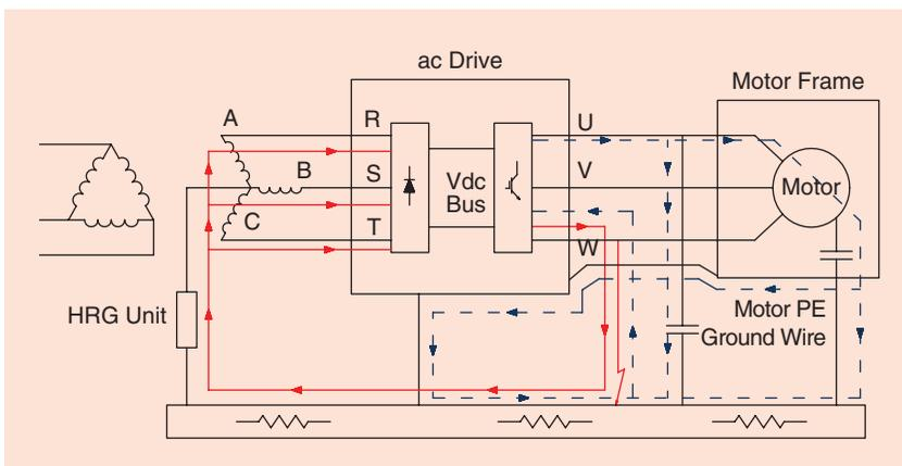
**FIGURE 11.** A UPS or ASD indicating a common mode current due to a switching supply and a zero sequence due to a ground fault on the load side.
