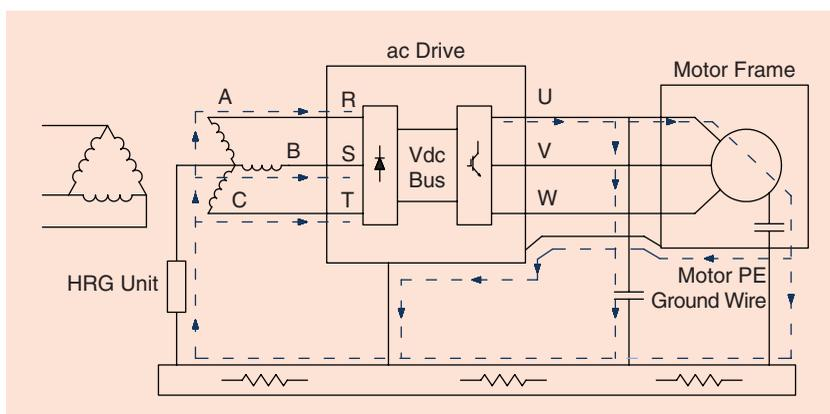
**FIGURE 8.** A UPS or ASD indicating common mode current due to switching supply. PE: protective earth.
