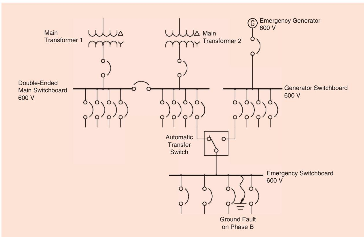
**FIGURE 2.** A single-phase fault scenario.
