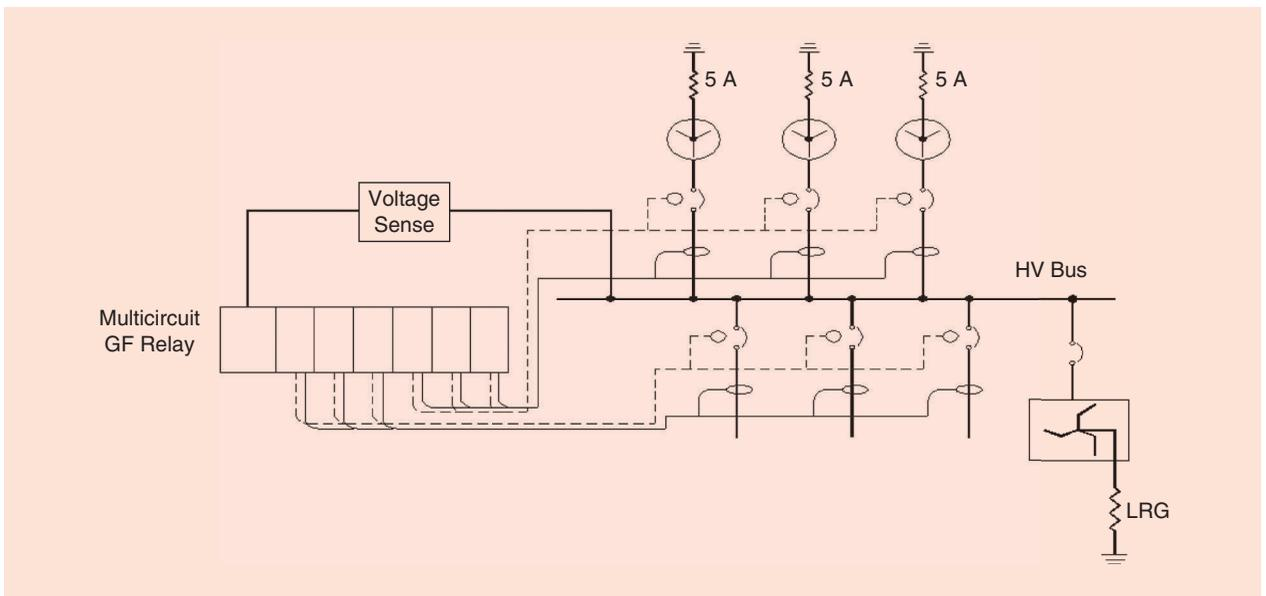
**FIGURE 7.** An extended MV hybrid system. HV: high voltage.
