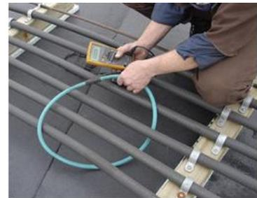
Navigation to the faulted device can be assisted by the use of fault tracking equipment (tracking signals or pulses impressed on the ground system and the use of hand held sensing equipment).
