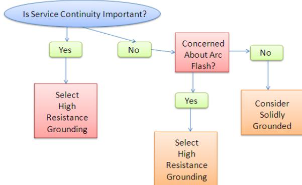
the proper application of High Resistance Grounding.
