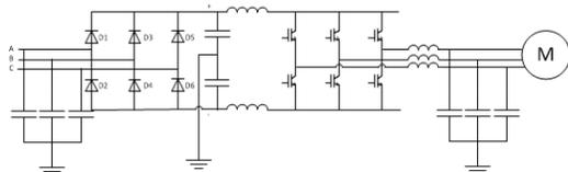
The additional capacitors are used to filter all undesired frequencies. What these additional capacitors do is provide alternate paths for ground fault currents to return. It may seem like a trivial amount but when you multiply the quantity of ASDs in a facility with a small amount of leakage current contribution by every ASD, it becomes a
