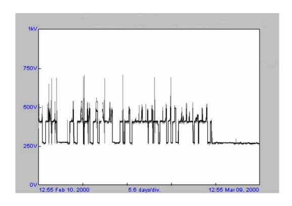
485 events with peak voltage above 700 volts due to intermittent ground faults.
