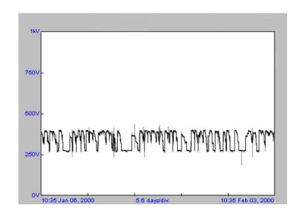
Transients controlled 0 peak events over 700 volts Peak voltage 660 volts
