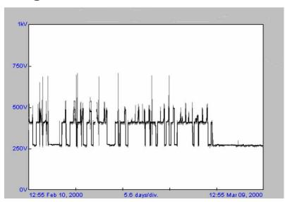
High level of transients 485 peak events over 700 volts Peak voltage 1050 volts
