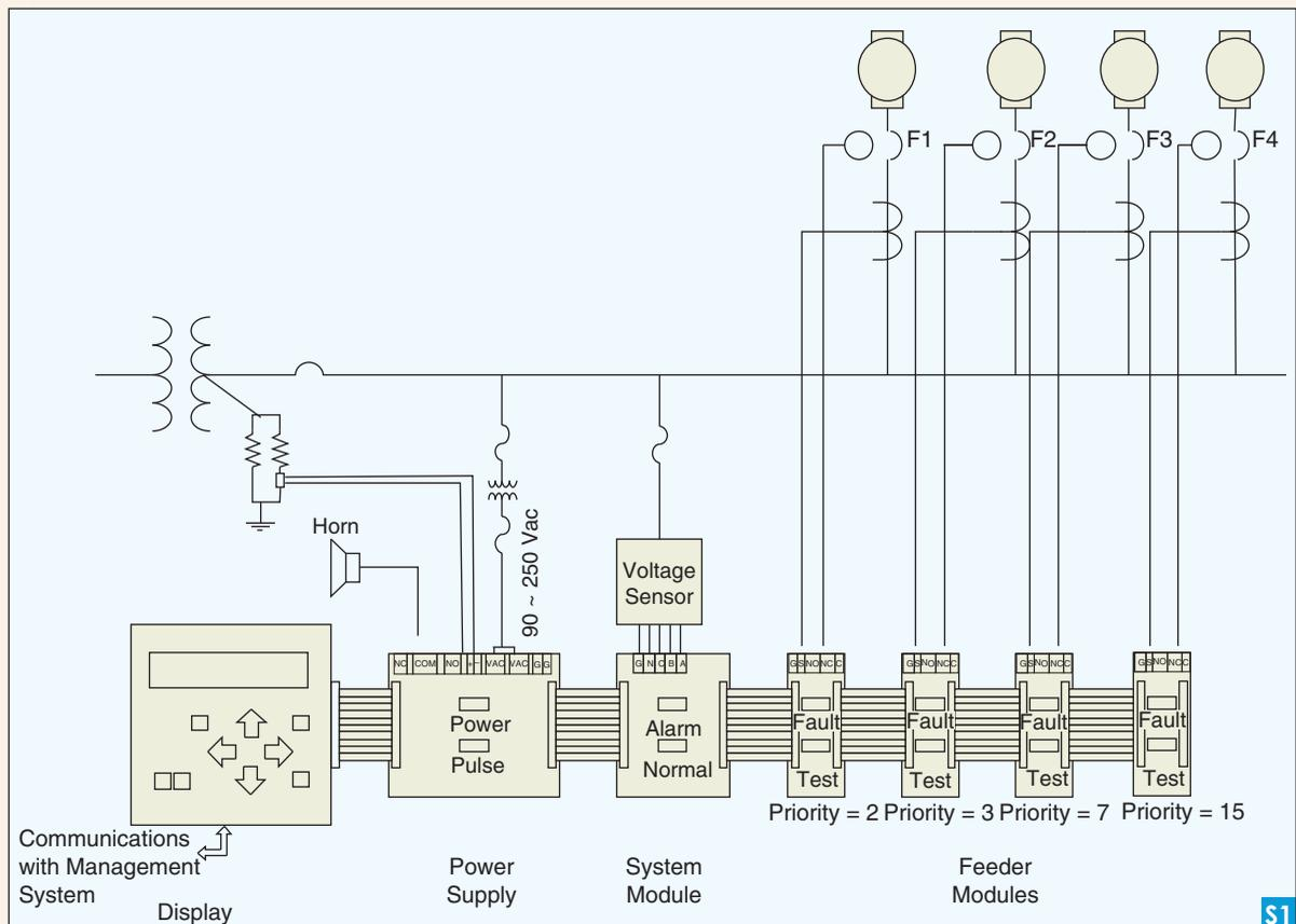
An HRG system with second fault protection.
