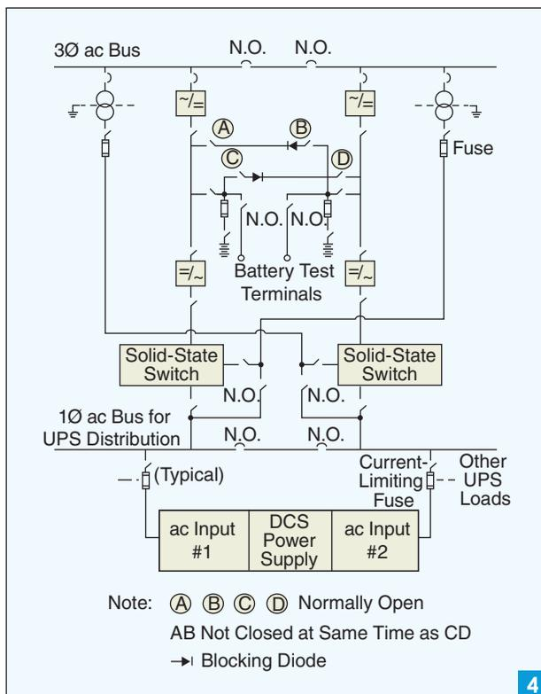
**An ac uninterruptible supply system configuration.**
