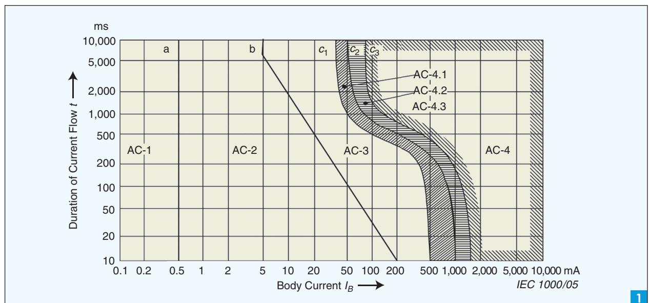
Conventional time/current zones of effects of ac currents (15–100 Hz) on persons for a current path corresponding to left hand to feet [1].
