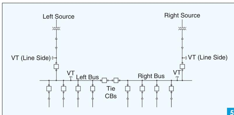
**A representative double-ended substation with two tie circuit breakers in series.**
