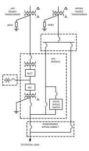
It is recommended that the bypass and inverter output sources be grounded same way, either solidly grounded or HRG. Typically, if the building distribution system is HRG, then the UPS inverter output should also be high resistance grounded. In this way, a ground fault in the critical load would not result in a transfer to bypass, but merely produce an alarm.
