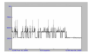
The graph shows the phase voltage readings from a 347/600V ungrounded automotive facility with high level of transients, peak voltage of 1050V and 485 events over 700V.
