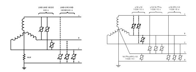
In a typical 3-phase 4-wire system a MCOV of 420V is sufficient for MOV's connected Line-to-Ground on a 347/600V system as the actual voltage does not exceed 347V and the TVSS is manufactured with this rating in mind.
