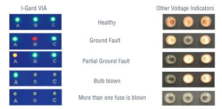
Table 1: shows all possible conditions that can be displayed using the LED lamps.
